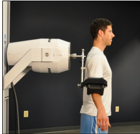
Align the shoulder with the axis of rotation of the shaft
