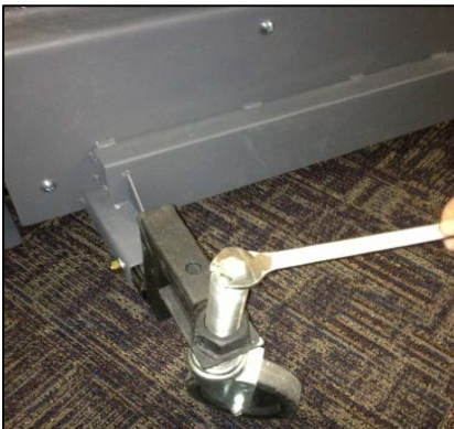
Figure 30 - Raise Casters to Lift Frame
