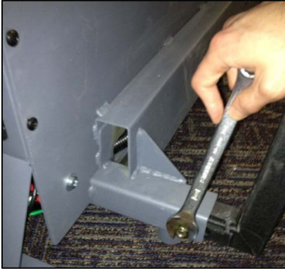
Figure 29 - Attach Caster to Frame
