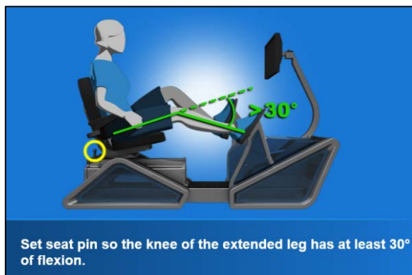
Figure 4 - Correct 30° Flexion Position
