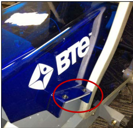
Figure 13 - Console Frame Screws
