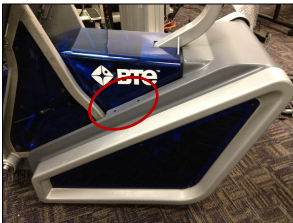
Figure 18 - Console Screw Attachments
