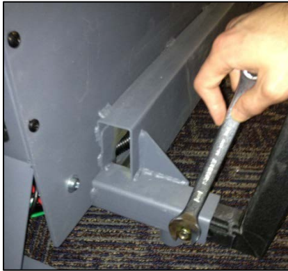
Figure 29 - Attach Caster to Frame
