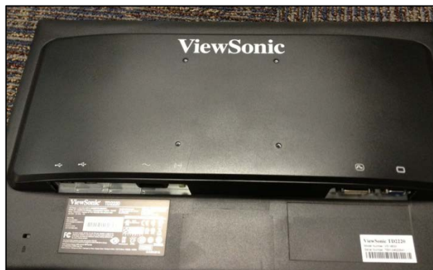
Figure 6 - Display with Screws Removed
