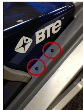
Figure 19 - Console Screw Attachments
