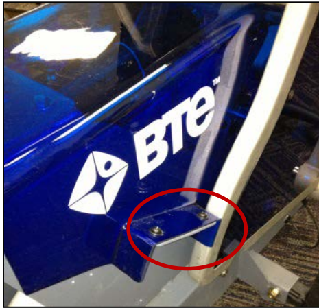
Figure 13 - Console Frame Screws
