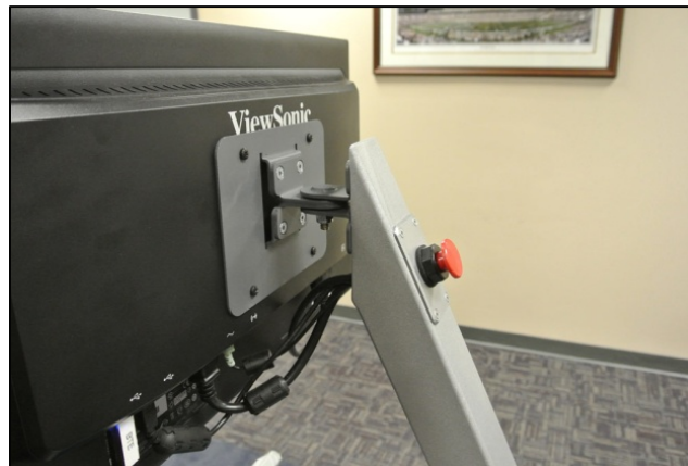
Figure 24 - Monitor Arm E-Stop
