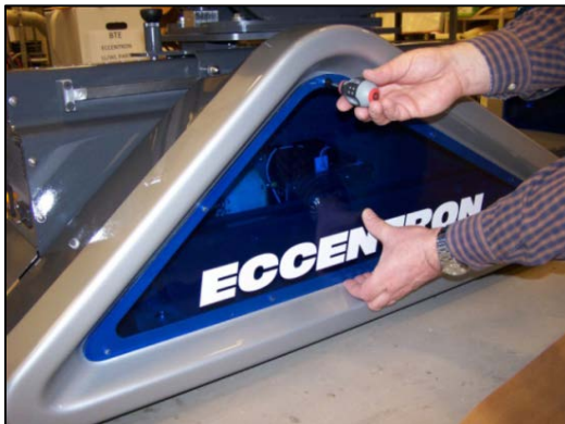
Figure 25 - Side Panel Screws
