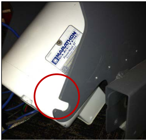
Figure 14 - Steel Mounting Hooks
