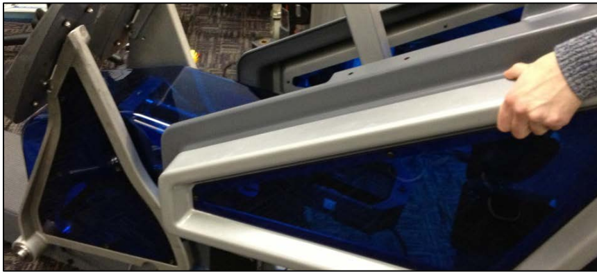
Figure 17 - Lower Console onto Frame
