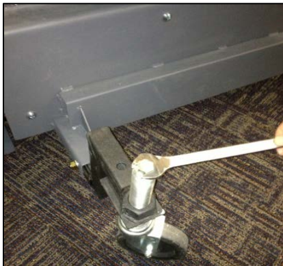
Figure 30 - Raise Casters to Lift Frame
