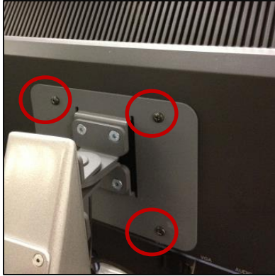
Figure 7 - M4 x 10 screws
