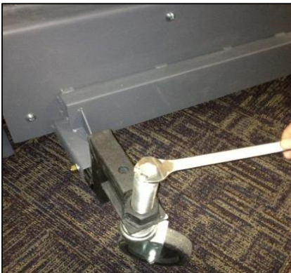
Figure 30 - Raise Casters to Lift Frame
