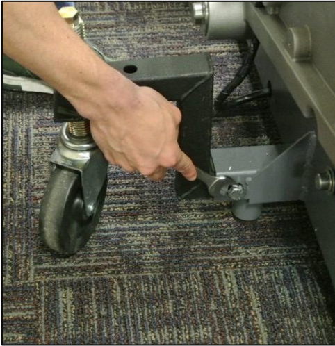
Figure 3 – Unscrew Tube Screw
