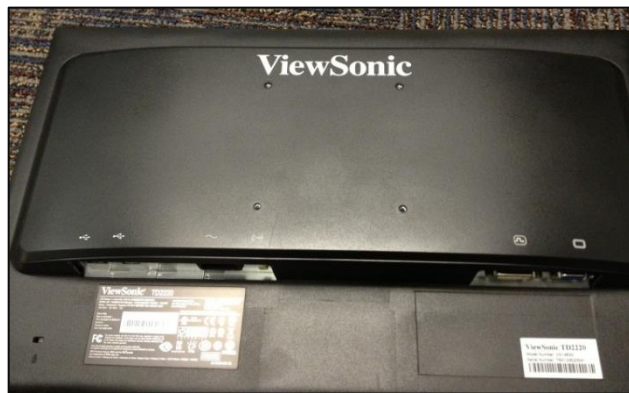
Figure 6 - Display with Screws Removed
