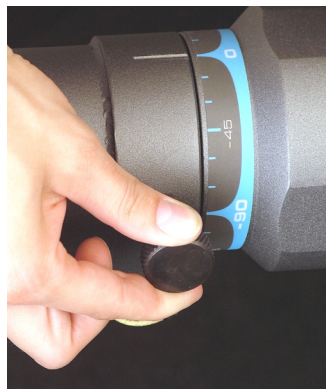
Figure 8-7. Turn the Retractable Pin
