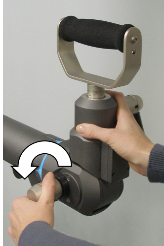
Figure 9-9. Loosen Bottom Retractable Handle
