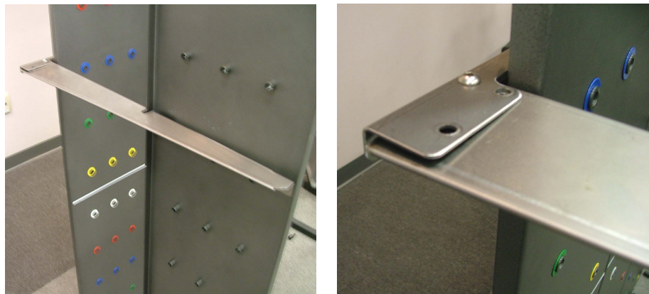
Figure 1-18. Position the Panel 6 Bracket and Secure It to the Back Bracket
