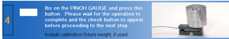
Figure 6-8. Pinch Gauge - Set the Weight
