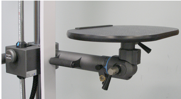
Figure 9-24. Secure the Bottom Shelf to the CLC
