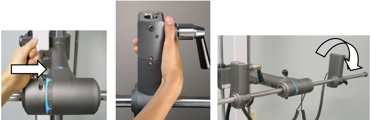
Figure 10-11. Rotating the UTM in the Sagittal Plane
