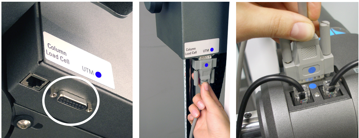
Figure 10-15. Connect the UTM to the Column
