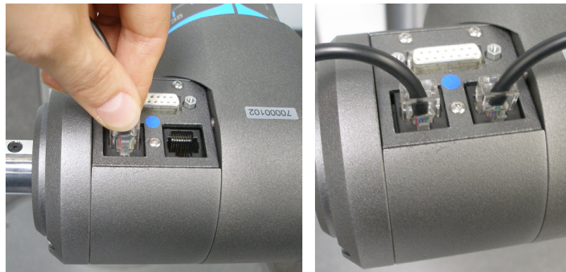
Figure 10-14. Attach the UTM Side Cables
