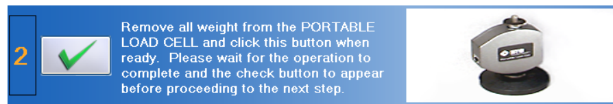
Figure 7-5. Portable Load Cell - Set the Zero Point
