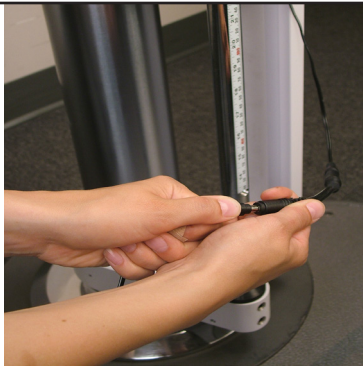
Figure 1-4b. Supply Power to the Column
