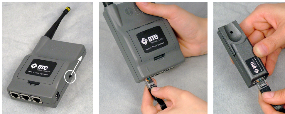
Figure 1-23. Connect a Tool to the Dock
