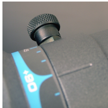
Figure 9-14. Lock Arm Retractable Pin
