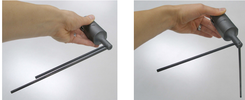
Figure 4-3. Check if Top Housing is Loose
