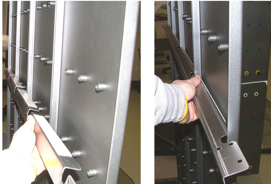
Figure 1-16. Position the Back Bracket and Adhere it to the FROM
