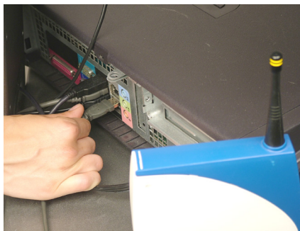
Figure 1-20. Attach Antenna and Plug Cable into Computer
