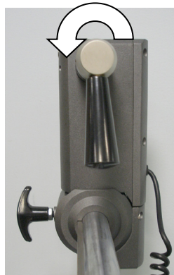
Figure 10-3. Loosen Top Retractable Handle
