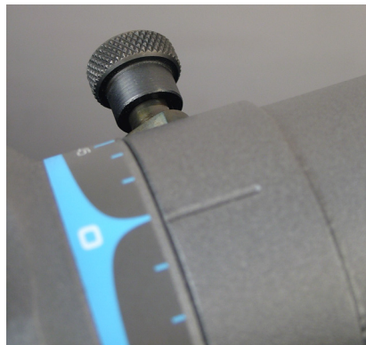
Figure 9-12. Unlock Arm Retractable Pin
