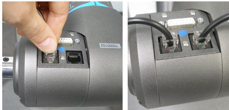
Figure 10-14. Attach the UTM Side Cables
