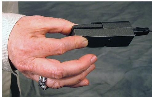
Figure 6-3. Pinch Gauge - Tip
