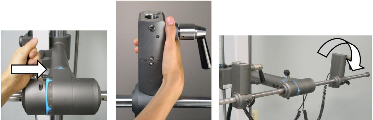
Figure 10-11. Rotating the UTM in the Sagittal Plane
