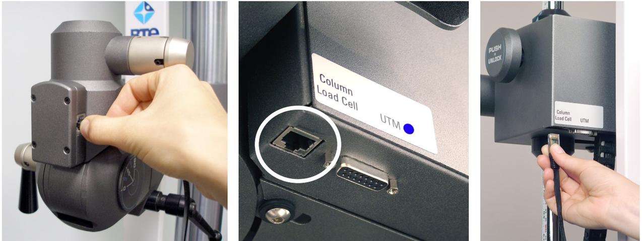
Figure 9-16. Connect the CLC to the Column
