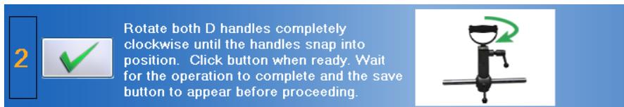
Figure 10-30. UTM - Set the Final Handle Rotation
