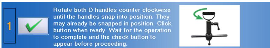
Figure 10-29. UTM - Set the Initial Handle Rotation
