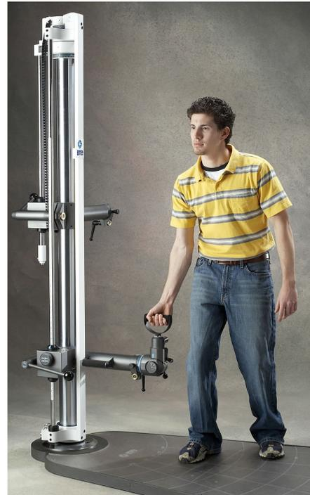
Figure 9-19. Sample Column Load Cell Isometric Strength Tests
