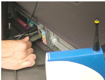
Figure 1-20. Attach Antenna and Plug Cable into Computer
