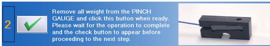
Figure 6-7. Pinch Gauge - Set the Zero Point
