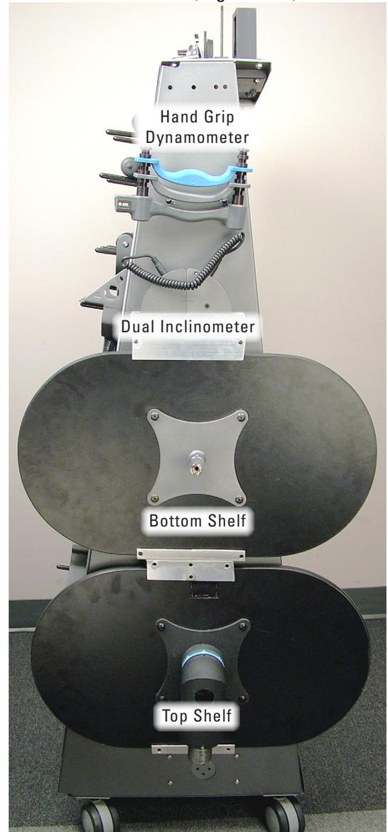
Figure 1-8a. Placement of Tools on Tool Rack - Front & Right Sides
