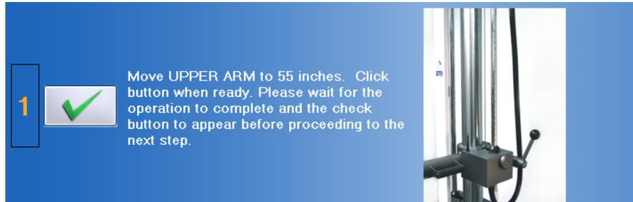
Figure 8-17. Column Upper Arm - Set the Initial Height
