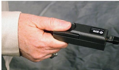
Figure 6-2. Pinch Gauge - Key
