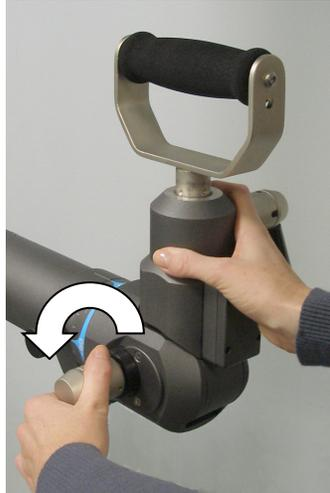
Figure 9-9. Loosen Bottom Retractable Handle
