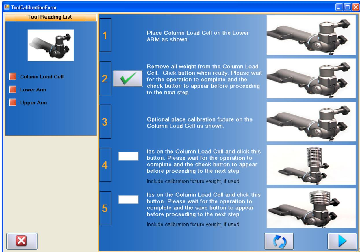
Figure 8-13. Column Load Cell & Column Arms Calibration Screen
