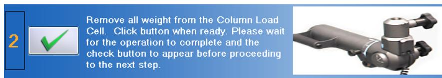
Figure 9-29. Column Load Cell - Set the Zero Point
