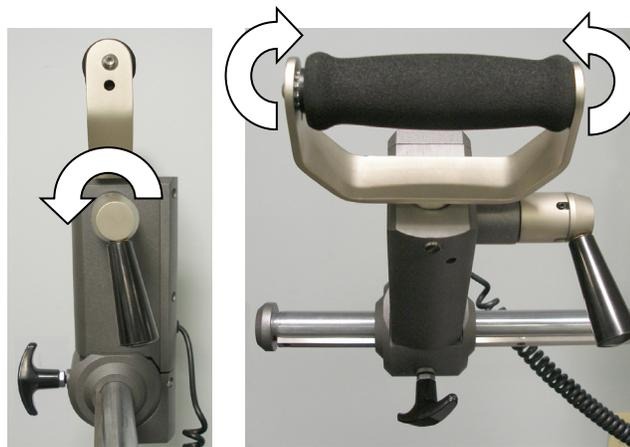
Figure 10-8. Rotating an Attachment in a UTM Side
