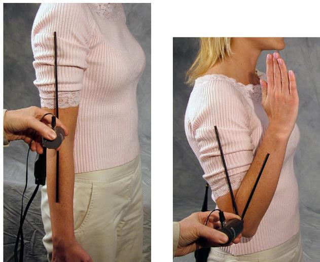
Figure 4-2. Example of Initial & Final Goniometer ROM Positions
