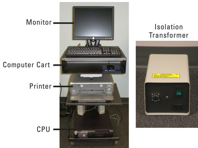
Figure 1-5. Computer Equipment and Cart
