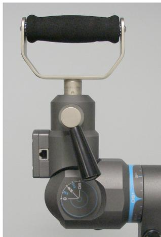
Figure 9-8. Handle Secured in CLC
