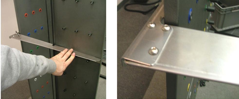
Figure 1-19. Adhering the Panel 6 Bracket and Securing All 3 Screws & Nuts
