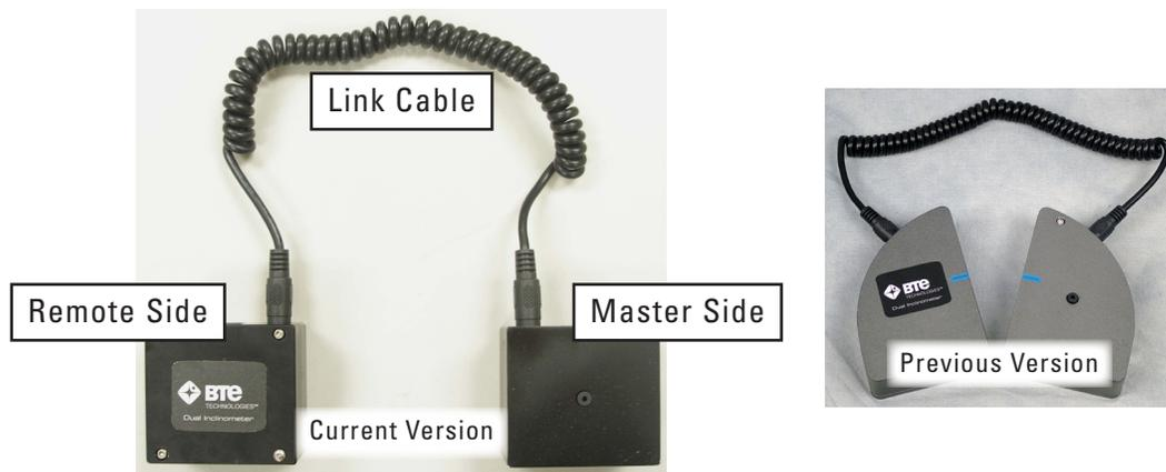
Figure 3-1. Dual Inclinometer - Current and Older Versions
