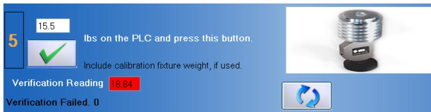
Figure 7-9. Portable Load Cell - Verification Failed
