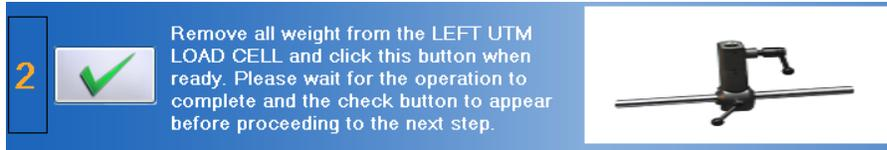
Figure 10-22. UTM - Set the Zero Point
