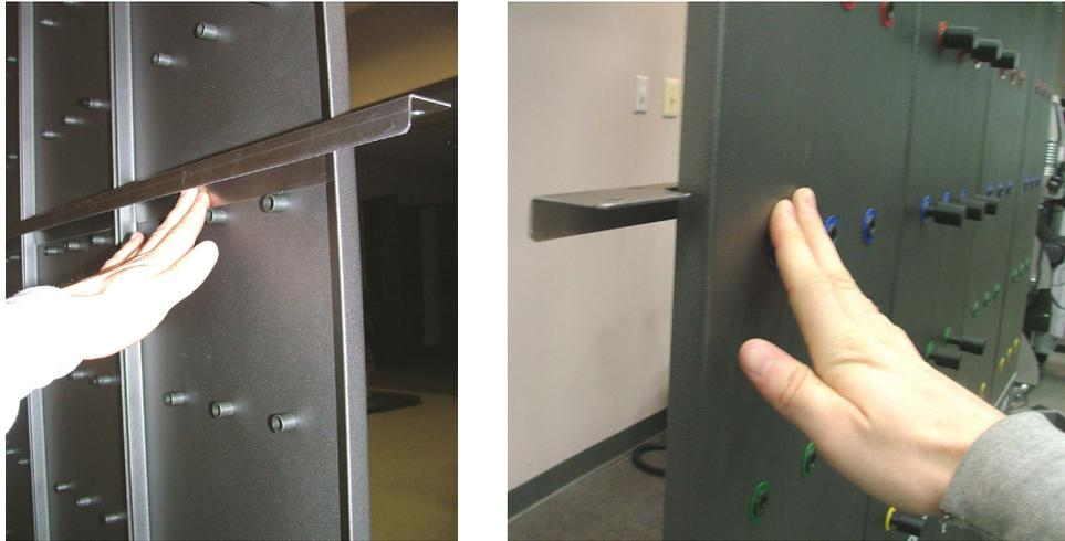
Figure 1-17. Secure the Back Bracket to Panels 1-4
