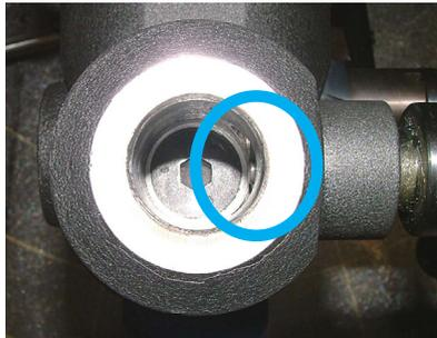
Figure 9-5. Top Retractable Handle Pin Not Visible
