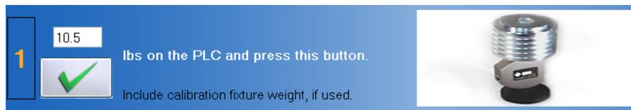
Figure 7-10. Portable Load Cell - Verify the Weight
