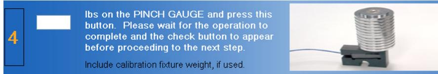
Figure 6-8. Pinch Gauge - Set the Weight
