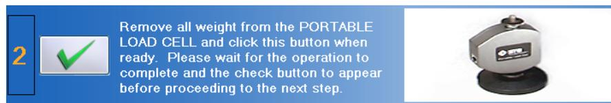
Figure 7-5. Portable Load Cell - Set the Zero Point
