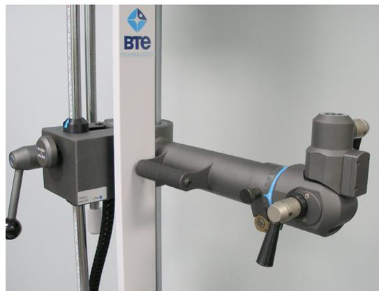
Figure 9-23. Secure the CLC to the Column Arm
