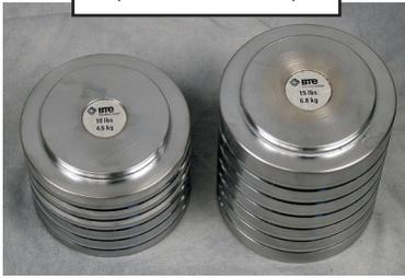
Hand Grip Dynamometer Calibration Fixture
