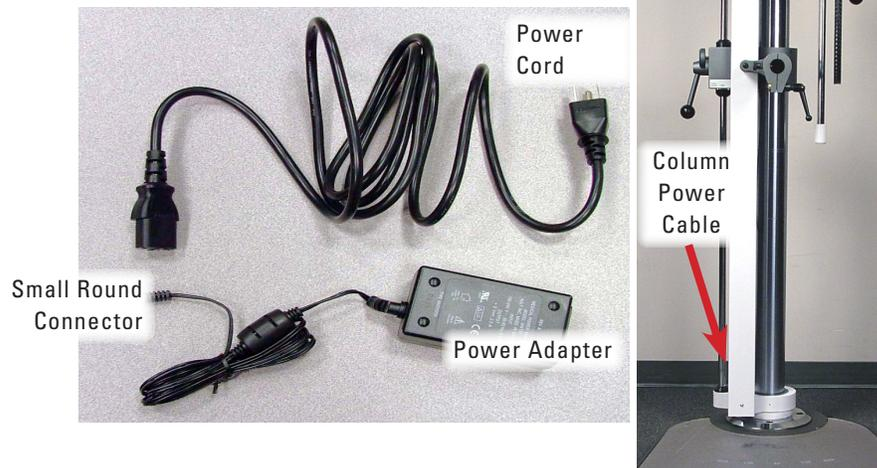
Figure 1-4a. Supply Power to the Column
