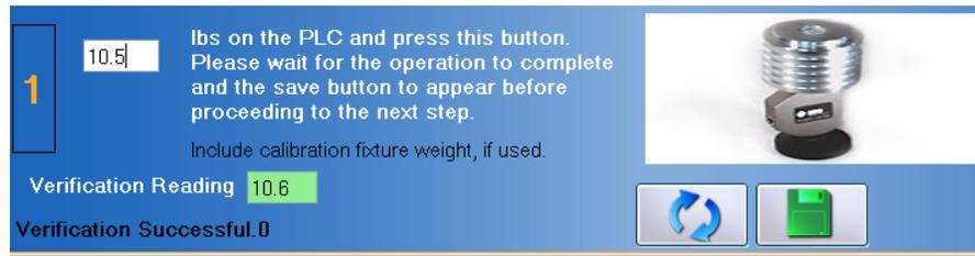
Figure 7-11. Portable Load Cell - Verification Successful
