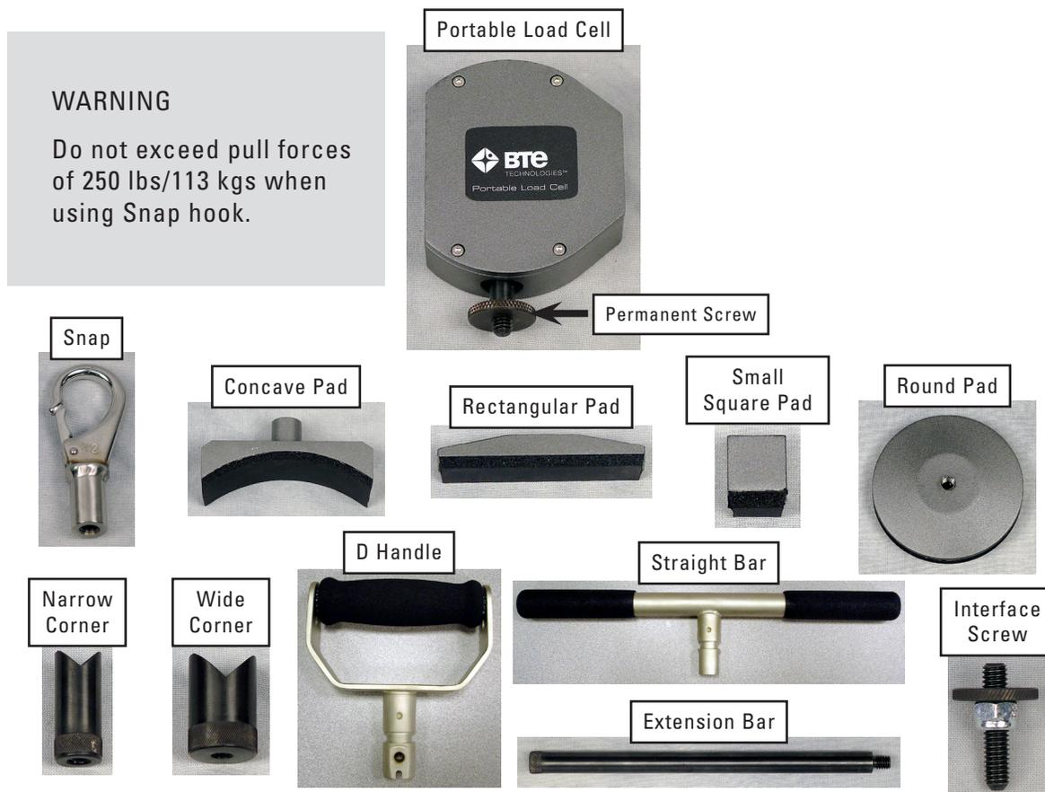
Figure 7-1. Portable Load Cell and Commonly-Used Attachments & Accessories
