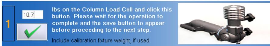
Figure 9-34. Column Load Cell - Verify the Weight
