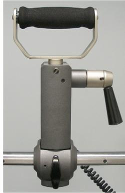
Figure 10-17. Attachment Secured to UTM Side
