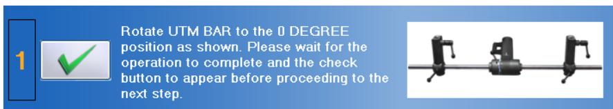
Figure 10-31. UTM - Set the Initial Bar Rotation
