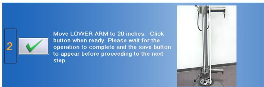
Figure 8-16. Column Lower Arm - Set the Final Height
