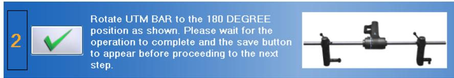
Figure 10-32. UTM - Set the Final Bar Rotation
