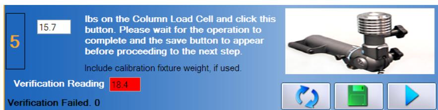
Figure 9-33. Column Load Cell - Verification Failed
