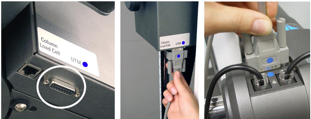
Figure 10-15. Connect the UTM to the Column
