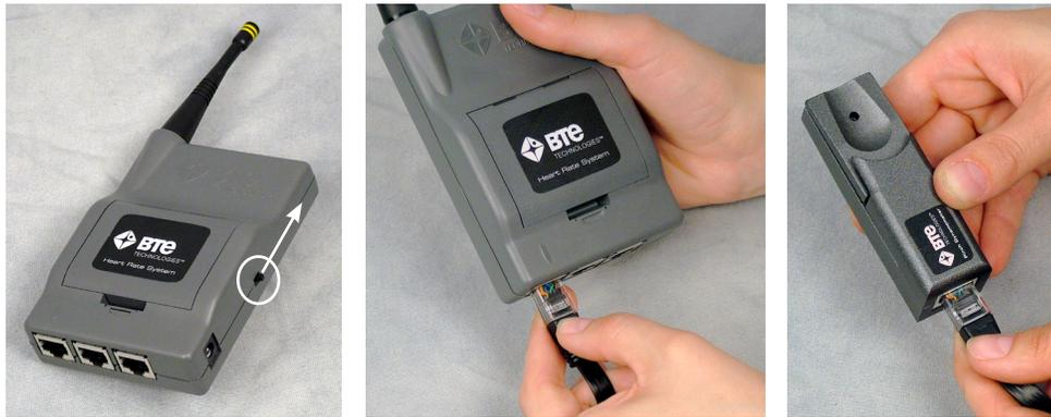
Figure 1-23. Connect a Tool to the Dock
