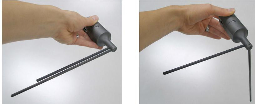
Figure 4-3. Check if Top Housing is Loose
