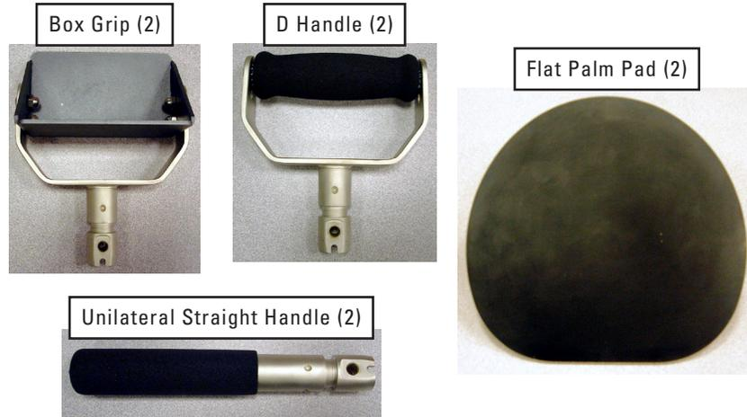
Figure 10-2. Commonly-Used UTM Attachments
