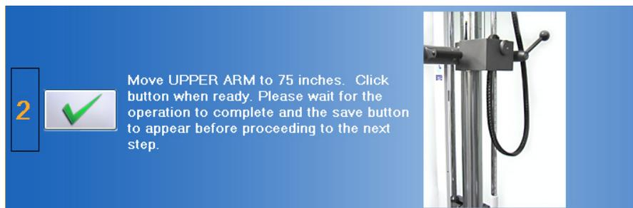
Figure 8-18. Column Upper Arm - Set the Final Height
