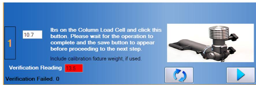
Figure 9-36. Column Load Cell - Verification Failed
