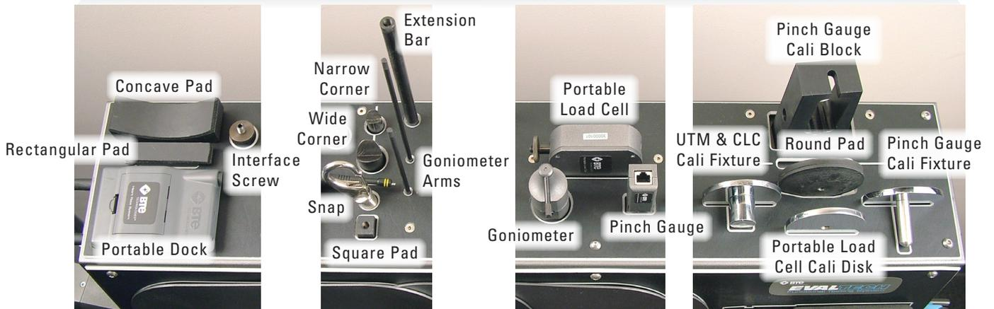
Figure 1-8c. Placement of Tools on Tool Rack - Top
