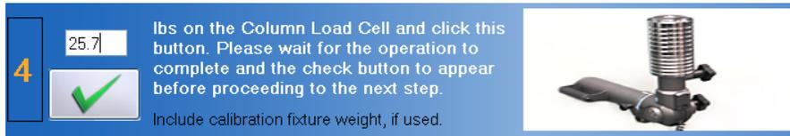
Figure 9-30. Column Load Cell - Set the Weight
