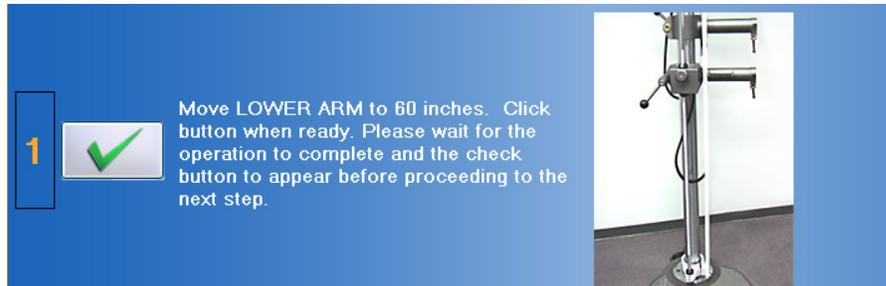
Figure 8-15. Column Lower Arm - Set the Initial Height
