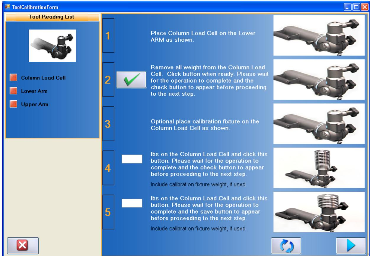
Figure 9-28. Column Load Cell & Column Arms Calibration Screen
