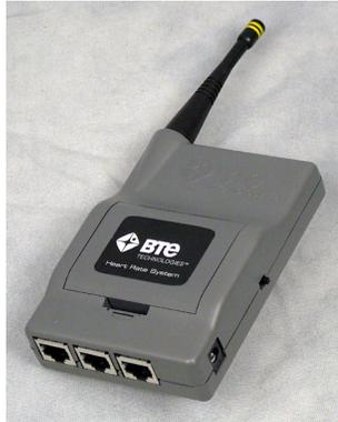
Figure 1-21. Attach Antenna and Insert Batteries
