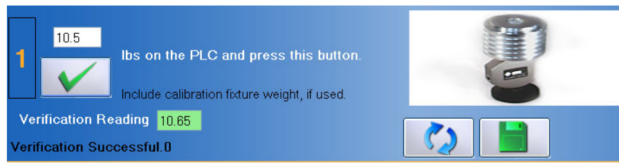
Figure 7-11. Portable Load Cell - Verification Successful
