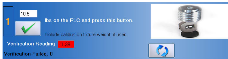
Figure 7-12. Portable Load Cell - Verification Failed
