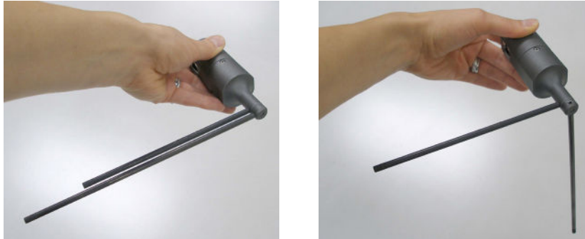
Figure 4-3. Check if Top Housing is Loose
