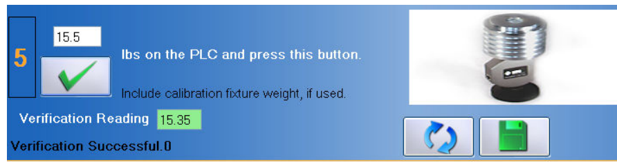
Figure 7-8. Portable Load Cell - Verification Successful
