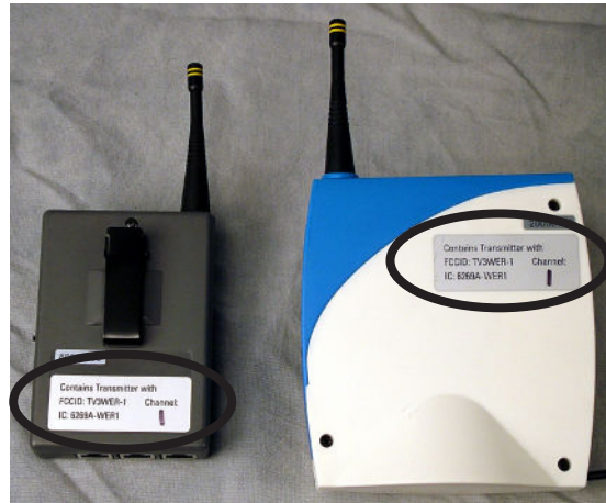
Figure 2-5. Verify Channel Numbers Match
