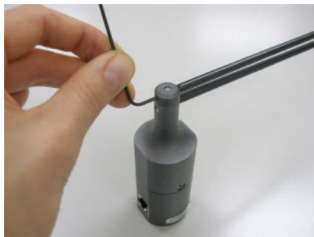
Figure 4-4. Tighten Set Screw
