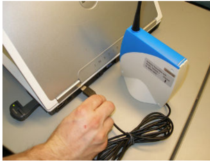
Figure 1-6. Attach Antenna and Plug Cable into Computer
