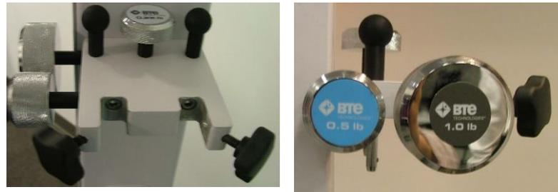
Step 3. Locate the head braces (also known as load cells) and secure them to the calibration plate.
