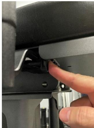
Step 8. Plug the power cord, which is located at the bottom back of the MCU, into the designated wall outlet. Hold your hand above the back of the MCU, next to the cable, and verify a light shines on your hand; this confirms the PCB is receiving power.
