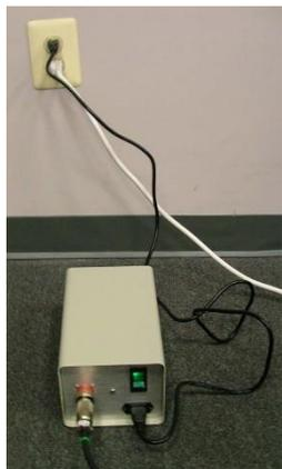
The use of extension cords is not recommended. If an extension cord cannot be avoided, use no less than 14-gauge wire. Keep the cord as short as possible, and use only hospital approved plugs. The extension cord MUST complete the ground from the MCU power supply cord to the wall outlet.
