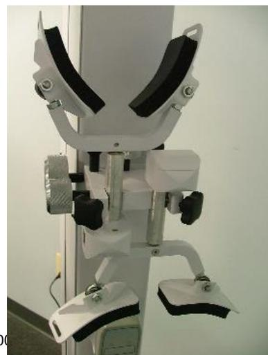
Step 5. Locate the calibration weights and calibration block and place them in the triangular bracket on the base.
