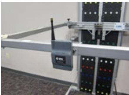
The PTK PLC is now ready to use for a Pull Test. When performing a pull test, the user should pull horizontally from the center axis of the load cell. Pulling at an angle not in line with the load cell axis will cause reduced readings.
