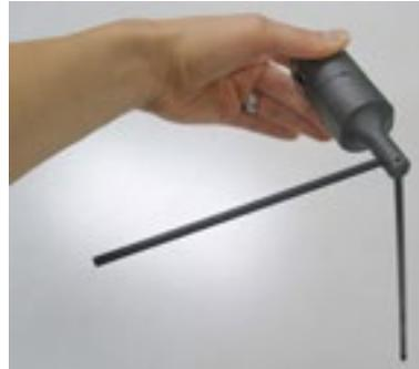
Step 2. Place the Goniometer in a horizontal position and position the arms parallel to the floor.
