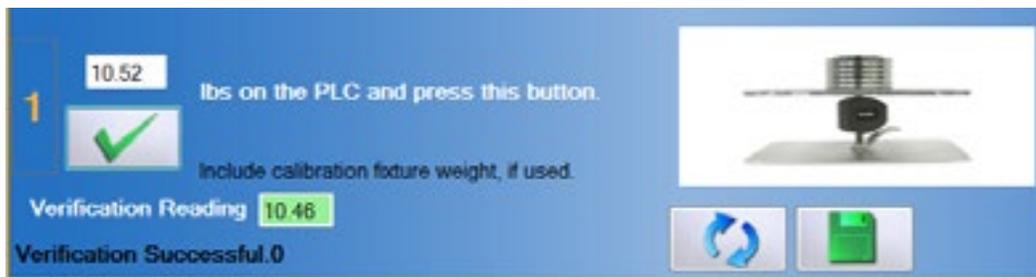
If the PTK Portable Load Cell was not properly calibrated, then the screen will say the verification failed and the measured weight will be in a red box. You may try re-verifying the weight or re-calibrating the tool until the verification is successful
