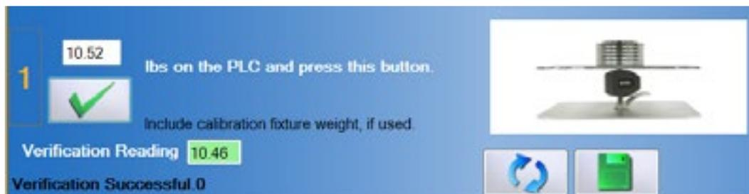
If the PTK PLC was not properly calibrated, then the screen will say the verification failed and the measured weight will be in a red box. You may try re-verifying the weight or re-calibrating the tool until the verification is successful.
