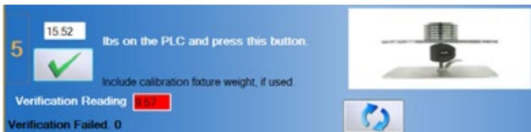
Step 11. Once the tool has passed verification, click on
