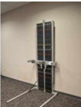
The PTK system weighs approximately 125 lbs. When moving the system, it is recommended that two or more people are used to safely lift the PTK.
