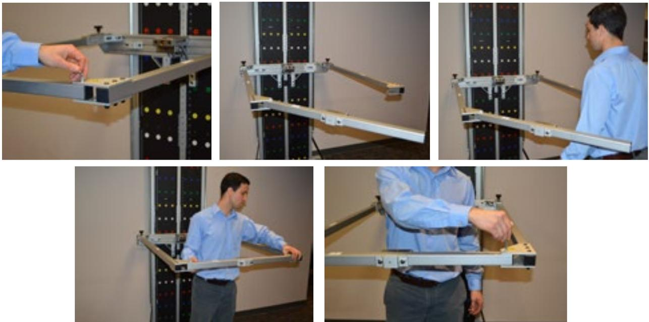
7) To remove the Pull Test Frame Attachment, simply unscrew and remove the Pull Test Frame Attachment Locking Knobs located on the Carriage. Lifting up gently on the attachment while unscrewing may allow for easier removal. Place the Pull Test Frame Attachment Locking Knobs into the Holding Brackets of the Carriage.
