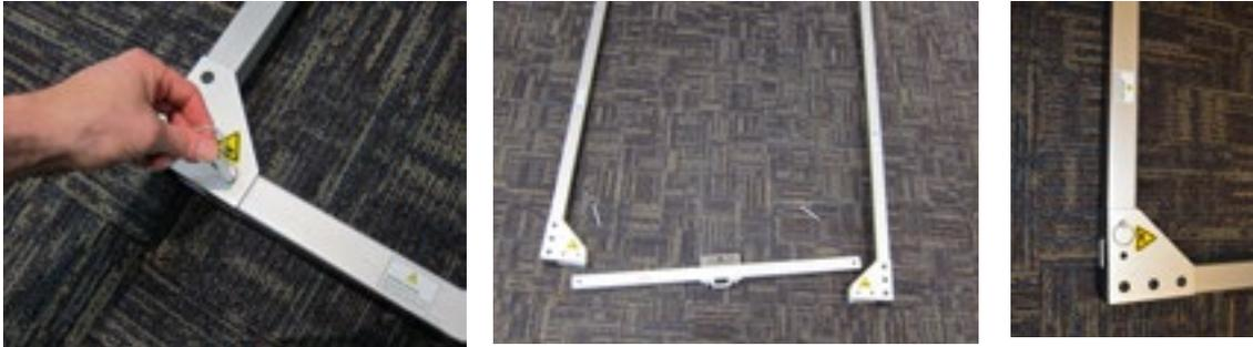
3) Locate the two Pull Test Frame Attachment Locking Knobs. If the Pull Test Frame Attachment Locking Knobs are secured into the Receiving Tubes of the Carriage, unscrew them, remove them from the receiving tubes, and place them into the Holding Brackets of the Carriage.
