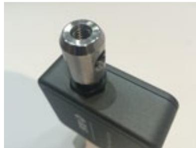
3) Take the PTK PLC and screw it onto the Platform in a clockwise rotation. The PTK PLC should be spun onto the Platform until the shaft bottoms out in the Platform Hub and is restrained from moving.
